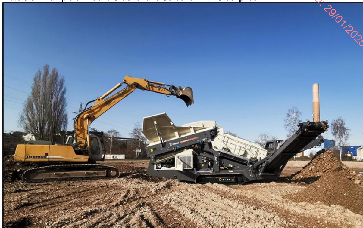
Plate 3-3: Example of Mobile Crusher and Screener with Stockpiles
